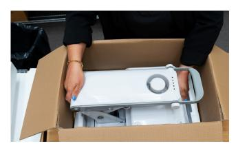
Place the press in the box carefully, ensuring that the press sits on the bottom foam completely.
